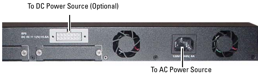
Figure 1-15. AC and DC Power Connection to Switch
